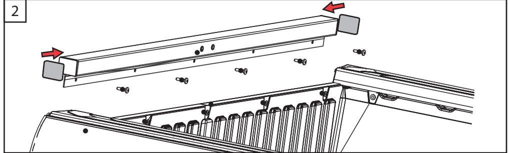
1 & 2. Using a T30 torx driver, remove the 5 fasteners securing the header rail to the bulkhead at the front of the bed. Adhere the gasket to the header rail end caps and reinstall the header rail.
