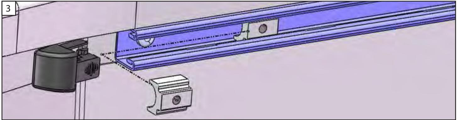
3. Slide the clamp assembly (3 per side) into the Utility rail, position one front, one center and one rear.
