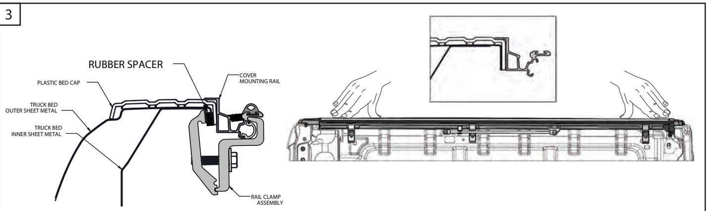
3. Using three (3) clamps per side attach the rail to the bed, position the clamps adjacent to each of the black rail spacers. Apply downward pressure to the rail when tightening each clamp to ensure the rail sets flush and seals properly. A second set of hands may help. Figure 3. (Tip: Mount the center clamp first but do not tighten completely. This will give you the ability to adjust the rail as the outer clamps are attached)
