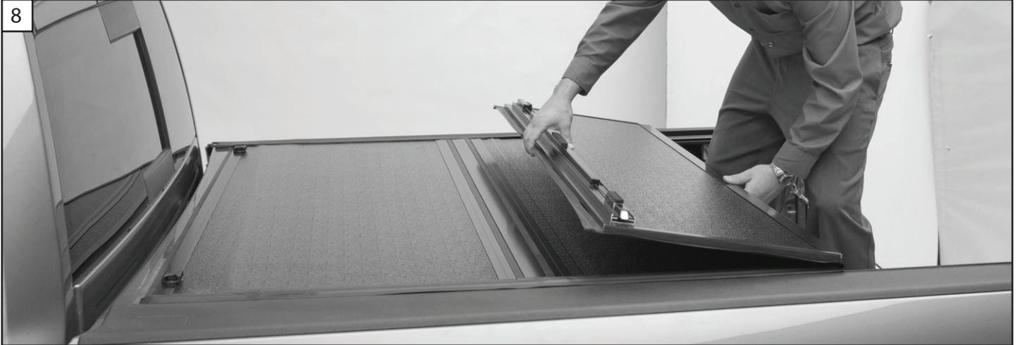
8. Carefully unfold the cover. Position the cover so it is centered side to side and front to back on the truck bed.
