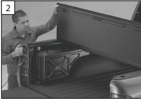
1 & 2. To open the cover: Lower the tailgate and pull the cable. While pulling on the cable lift the panel up and towards the cab.
