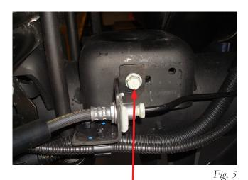
Remove bolt holding bracket
