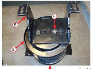
Fitting side of air spring assembly
