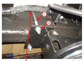
Do not pinch the wiring harness when installing the U-bolt
