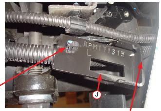
Insert tab on ABS wire loom here
