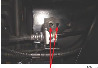
Align brake/ABS bracket hole and tab with holes in the lower bracket
