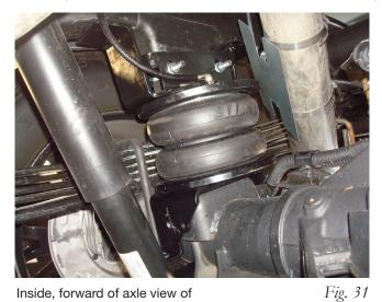
Inside, forward of axle view of driver's (left) side installation.
