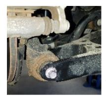
5. Install fitting (G) in the air spring (D). Tighten fitting 1 1/2 turns beyond hand-tight. Install roll plate (E) and lower air spring bracket (F) with two M10-1.5 x 25 hex cap screw bolts (I) and two M10 split lock washers (H) (Fig. D.28). Torque M10 bolts to 46Nm (34 lb.ft.).
