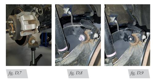
3. Support rear knuckle with jack (Fig. D.7). Remove rear upper control arm outer pivot bolt (Figs. D.8 & D.9).
