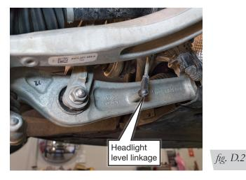
For cars equipped with auto-leveling headlights, installers must purchase the Air Lift Performance kit 33127. The new headlight linkage is shorter than the factory linkage. 5. Remove the lower pinch bolt on the fork mount (Fig. D.3).
