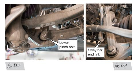
6. Remove the sway bar end link from the fork mount (Fig. D.4).
