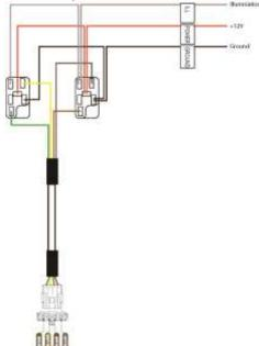
**Illumination (Gray)** - This wire provides power to the switch lights. It should be hooked up to a light circuit in the vehicle (dash lights) or it can be hooked up to a 12 volt switched source.
