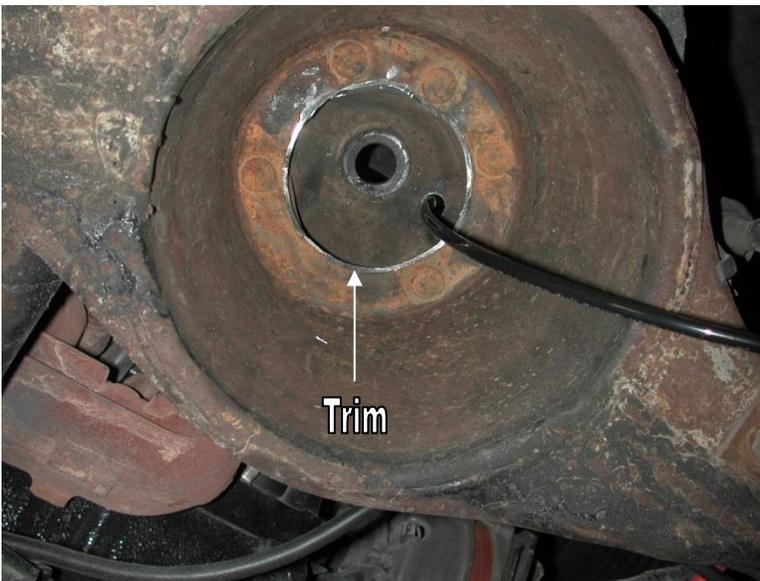
3. The upper coil spring retainer may need to be trimmed to clear the top of the CoilOver.
