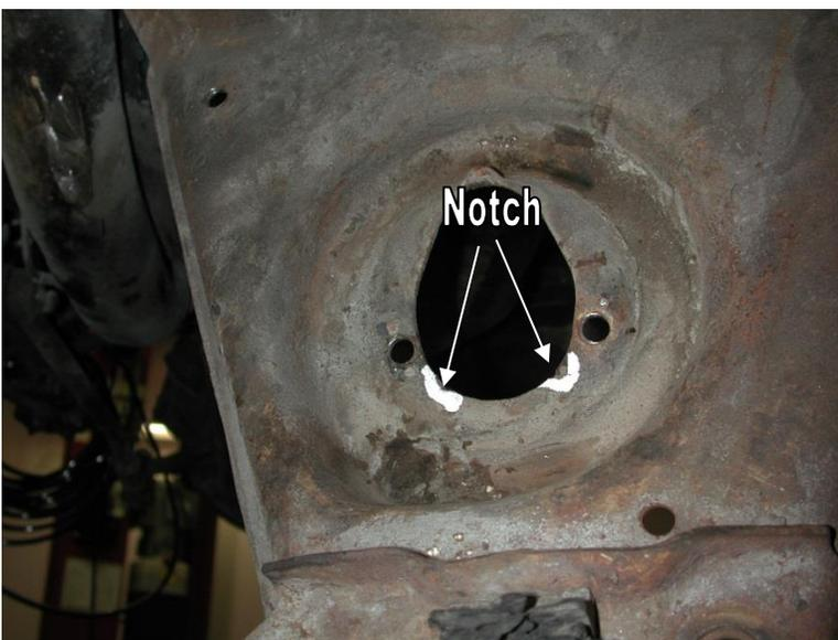
7. Two notches must be made in the lower arm for shock clearance.
