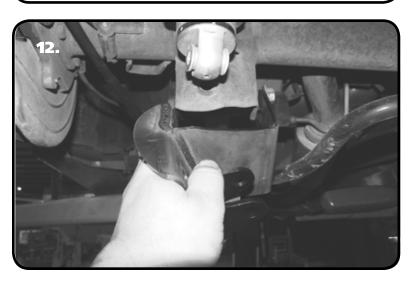
**12.** Slide the Lower Shock mount on to the Axle Mount. The Shock Mount wraps around the OEM Control Arm mount. The Slots on the side of the Mount slide on the Lower Control Arm Mounting Bolt. Install (1) 3/8-16 x 1 1/4" bolt (Threads pointing forward) through the hole in the Shock Mount and Lower Control Arm Mount. Install a 3/8" Flat Washer and 3/8" Nylok Nut on the Bolt and tighten. Tighten the Lower Control Arm Bolt.
