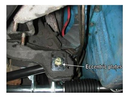
10. Attach the other end of the lower control arm to the factory frame mount using a  $\frac{1}{2}$ " x 4  $\frac{1}{2}$ " bolt and Hex nut.
