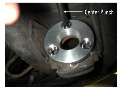
5. Using the bushing retainer as a template, mark the holes to drill with a center punch.
