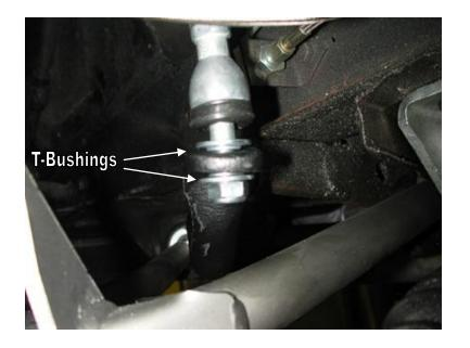
4. Slide a T-bushing over the straight end of the PosiLink, then slide it through the sway bar. Another T-bushing will be installed on the bottom along with a 10mm Nylok nut.
