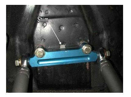
1. Bolt the upper StrongArm to the body using  $\frac{1}{2}$ " x 2  $\frac{1}{2}$ " bolts, flat washers and lock washers. A shim is supplied and may need to be installed between the body and the arms to achieve proper alignment.
