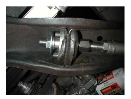
8. The bearing stud should already be threaded into the lower arm, factory set at 2-15/16" (measuring from the end of the arm to the bearing).
