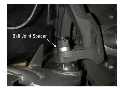
12. Slide the ball joint boot over the ball joint, then place the spindle over the ball joint stud. A ball joint spacer will be necessary to align the castle nut with the cotter pin hole. Grease ball joint
