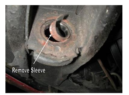
3. Be sure to remove the outer bushing sleeve from the strut rod frame mount.
