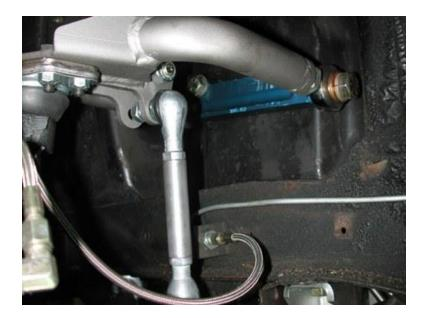
3. Attach the 90 degree end of the PosiLink to the rear tab of the upper control arm using a 10mm Nylok nut and a 3/8" flat washer on each side of the tab.
