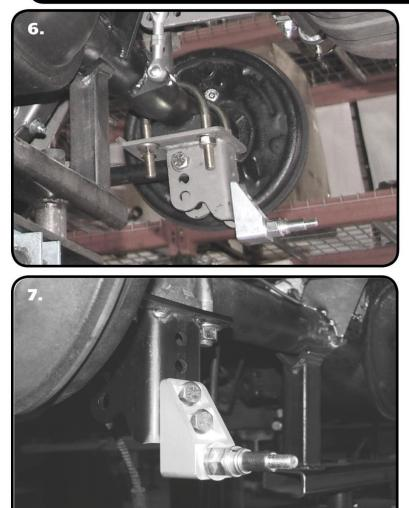
**6.** Install the Lower Axle Mount onto the Axle using the supplied U-Bolts. Run the nuts down to hold the mount in place, but DO NOT tighten yet.
