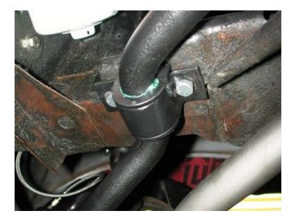
1. Apply lubricant to the poly bushing, then slide it over the sway bar.
