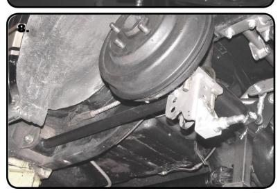
**8.** Install the Lower Bars. The Front Lower uses the WIDE(70013767) R-Joint Spacers inserted into each side of the R-Joint. The Axle end of the bar gets a NARROW(70013334) R-Joint Spacer inserted into each side of the R-Joint. The bar is attached to the Axle Mount in the **TOP HOLE** using (1) 5/8" x 2 3/4" Hex Bolt, and (1) 5/8" Thin Nylok Jam Nut. The front of the Lower Bar is attached with 1/2"x 6" Hex Bolt(64-67) or 1/2"x 4 1/2"Hex Bolt(68-70), and (1) 1/2" Nylok Nut.
