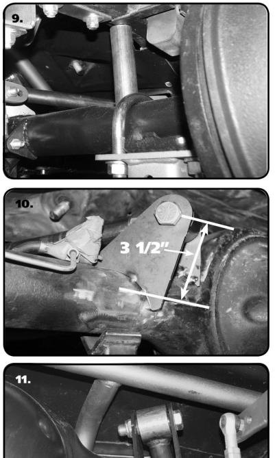
**9.** One helpful trick to maintain ride height when setting the pinion angle is to put a spacer between the axle and the frame. The spacer should be 4 1/2" tall. Set the pinion Angle and axle center. When measuring the axle center you can measure off of the frame rails. We also use a plum bob off the quarter panels to double check the axle center. Refer to Page 6 on Setting the Pinion Angle.
