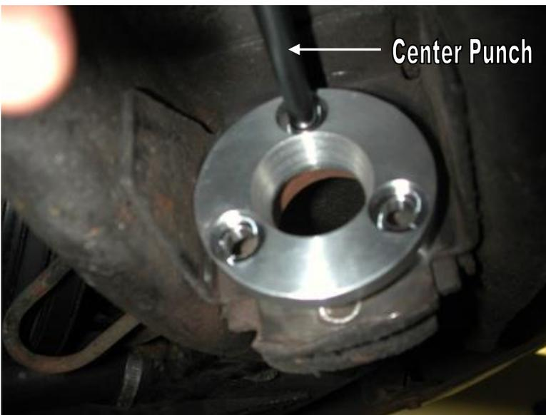
5. Using the bushing retainer as a template, mark the holes to drill with a center punch.
