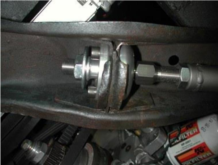
8. The bearing stud should already be threaded into the lower arm, factory set at 2-15/16" (measuring from the end of the arm to the bearing).
