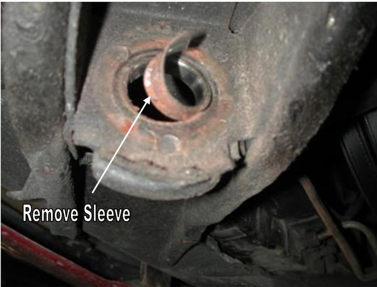
3. Be sure to remove the outer bushing sleeve from the strut rod frame mount.
