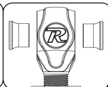
**New R-Joints will be quite stiff (75-90 in/lbs breakaway torque) until they "break in" after a few miles of use. After the break in period they will move much more freely. Because the composite bearing race contains self lubricating ingredients, no additional lubrication is needed or desired. Any additional lubrication will only serve to attract more dirt and debris to the R-Joint and actually shorten its life.**
