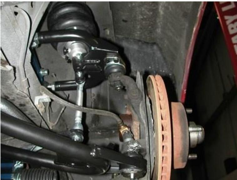
3. Bolt the upper arm to the spindle using the hardware and cotter pin supplied.
