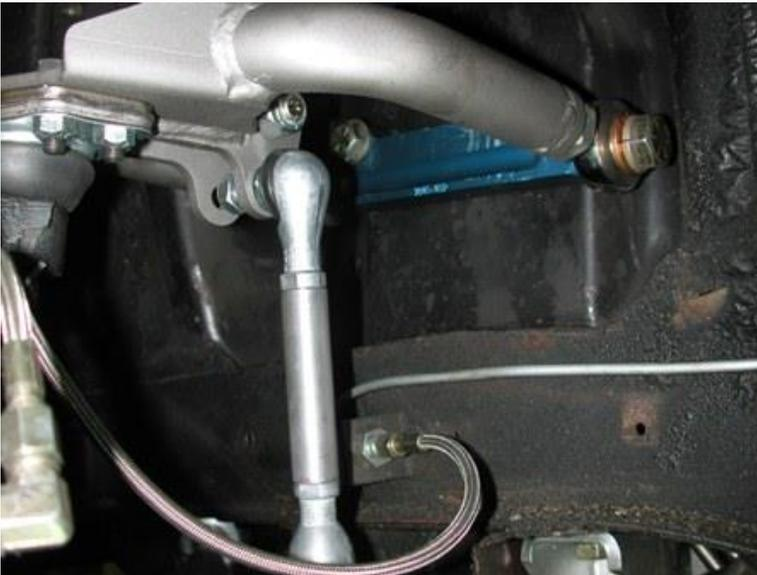
3. Attach the 90 degree end of the PosiLink to the rear tab of the upper control arm using a 10mm Nylok nut and a 3/8" flat washer on each side of the tab.
