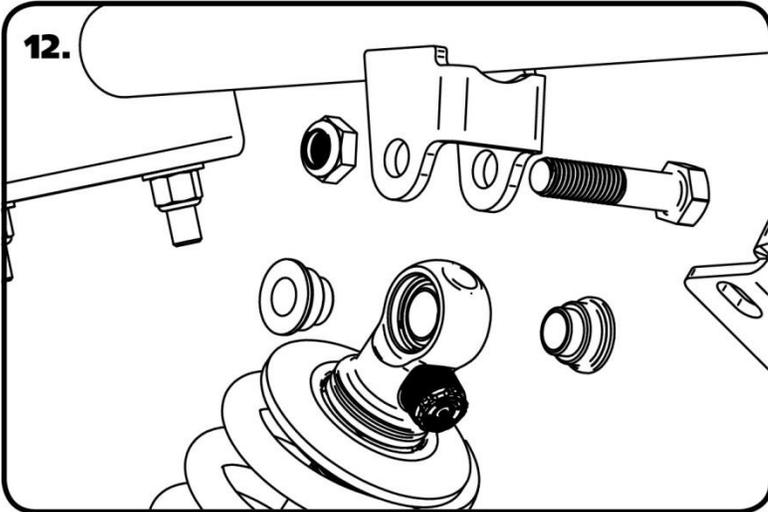
**Remove the Spacer from between the Axle and Frame.**
