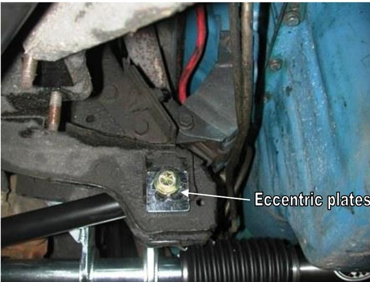
10. Attach the other end of the lower control arm to the factory frame mount using a 1/2" x 4 1/2" bolt and Hex nut.
