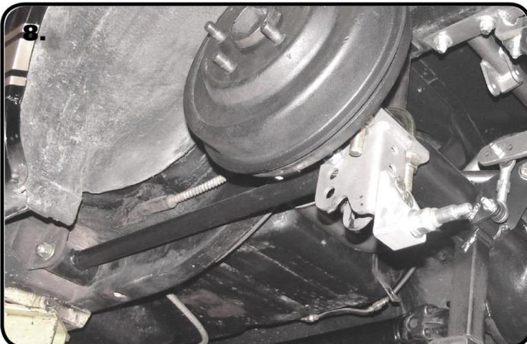
8. Install the Lower Bars. The Front Lower uses the **WIDE**(70013767) R-Joint Spacers inserted into each side of the R-Joint. The Axle end of the bar gets a **NARROW**(70013334) R-Joint Spacer inserted into each side of the R-Joint. The bar is attached to the Axle Mount in the **TOP HOLE** using (1) 5/8" x 2 3/4" Hex Bolt, and (1) 5/8" Thin Nylok Jam Nut. The front of the Lower Bar is attached with 1/2"x 6" Hex Bolt(64-67) or 1/2"x 4 1/2"Hex Bolt(68-70), and (1) 1/2" Nylok Nut.
