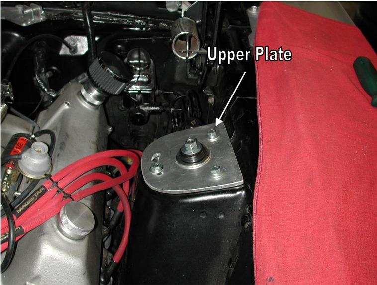
1. Place the upper plate on top of the strut tower. While holding the upper Shockwave mount up to the bottom of the strut tower, fasten the assembly with three 5/16" x 1" flange bolts.
