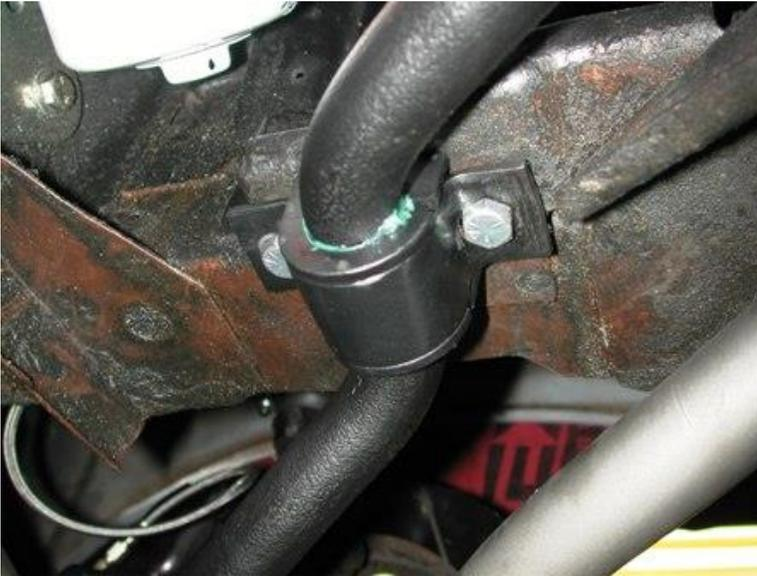
1. Apply lubricant to the poly bushing, then slide it over the sway bar.
