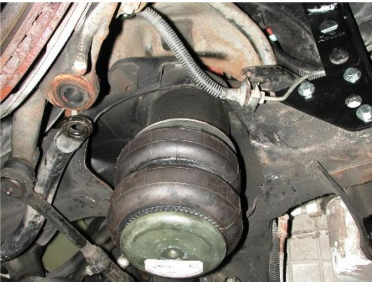
6. Place the air spring assembly into the coil spring pocket with the stud protruding through the OEM shock hole. Tighten with 7/16" Nylok nut and flat washer. The lower cup will just sit in the lower arm offsetting the spring towards the spindle.
