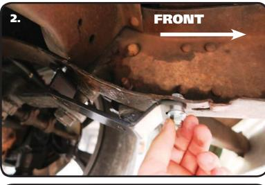
**2.** The MuscleBar Mount attaches to the frame using the holes from the OEM mount. The end of the frame bracket with the angled bends goes forward. Attach the bracket using a  $3/8"-16 \times 11/4"$  bolt, 3/8"-16 Nylok nut and a 3/8" Flat Washer on top and bottom. The same hardware setup is used in each hole. Repeat on the other side and tighten hardware.
