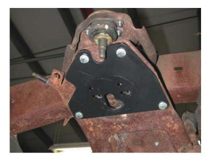
1. Hold the upper plate to the cross member as shown in the picture to the left and clamp to frame. Using the plate as a template drill four 3/8" holes in the cross member.
