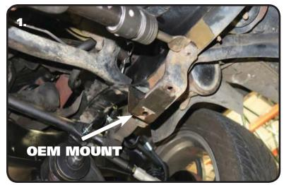
**1.** Some trucks are equipped with a OEM swaybar. If your truck has one, the OEM mount will need to be removed to install the MuscleBar. This is done by removing the rivets. The rivets can be removed by chiseling the heads off and driving them out or by drilling the rivets out. The new Frame Mount bolts directly in place of the old mount. If your truck doesn't have a sway bar, the mounting holes will still be in the frame.
