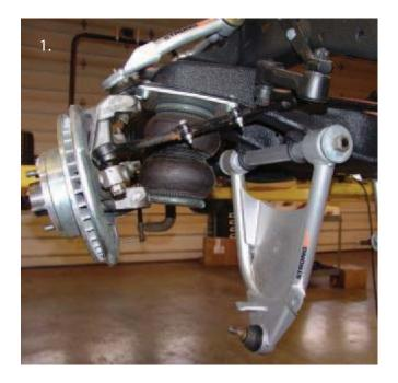
1. Bolt the lower Strong Arm to the frame using the OEM fasteners. The supplied cross shaft has 2 sets of holes. This CoolRide control arm uses the set of holes that are 8.705" center to center. **Image 2** illustrates the holes used. Make sure to align the dowel in the frame with one of the holes in the cross shaft that is 8.705" apart.
