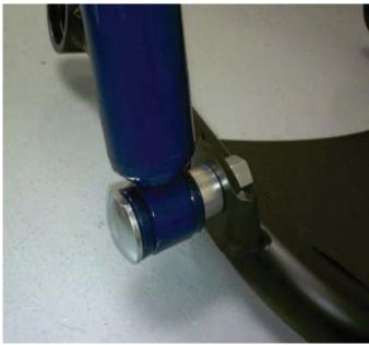
2. Attach the shock to the upper mount using the new rubber bushings and hardware supplied.
