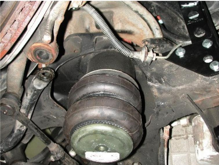
6. Place the air spring assembly into the coil spring pocket with the stud protruding through the OEM shock hole. Tighten with 7/16" Nylok nut and flat washer. The bottom of the air spring will attach to the lower arm using a 3/8" x 3/4" bolt, lock washer and flat washer.
