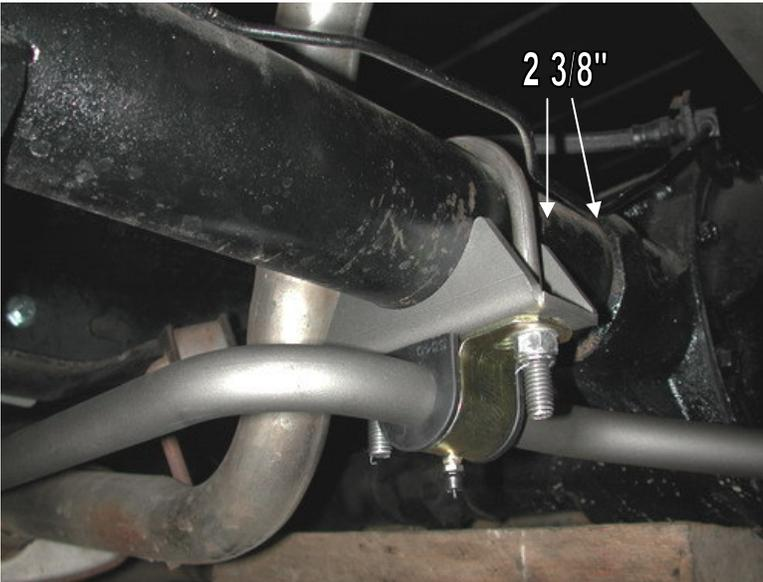
5. Attach the axle bracket, bushing and bushing bracket to the axle using the U bolt, 7/16" Nylok nut and flat washers supplied.
