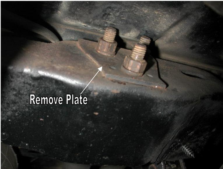
1. Loosen the 3 nuts holding the upper bar bracket to the cross member on the passenger side of the car. Remove the reinforcement plate.
