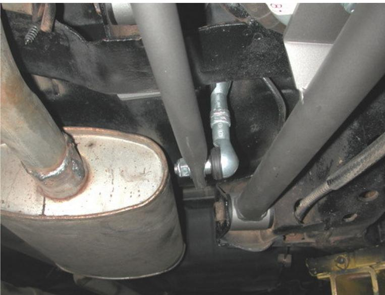
7. Attach the sway bar to the PosiLink using a 10mm Nylok nut and two 3/8" flat washers.
