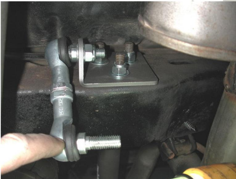
3. Most cars do not have an upper bar on the driver side, but the 3 bolt holes are there. 7/16" x 1 1/4" bolts, flat washers and Nylok nuts are supplied to fasten the bracket to the frame.
