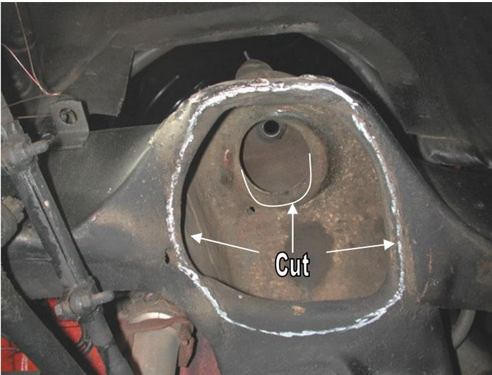
2. The inside lip of the pocket must also be removed to allow for Shockwave bellow clearance.
