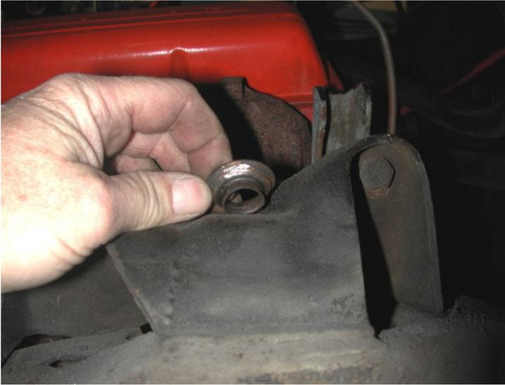
4. Surrounding the hole that the factory shock stem went through is a bushing cup. This must be removed using a chisel or air hammer.
