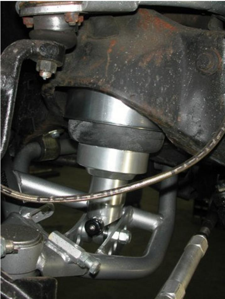
6. Insert the Shockwave into the coil spring pocket with the stud sticking through the factory shock hole. See assembly diagram on next page.
