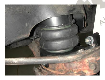
2. The coil spring pocket will need to be trimmed for air spring clearance as shown in the picture.
