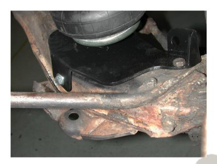
1. Place the lower air spring plate onto the lower control arm as shown in the picture. This is the Drivers side with the shock mount to the rear of the control arm. The plate will index off the rear strut arm bolt. The other two holes must be drilled for 3/8" x 1 1/4" bolts. Install flat washers and Nylok nuts.
