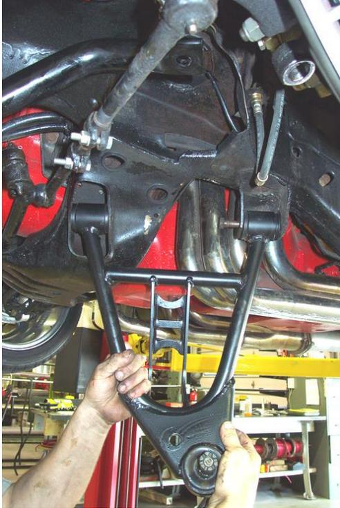
1. After removing the factory lower control arm, clean the bushing mounting surfaces on the frame and lubricate with lithium grease.
