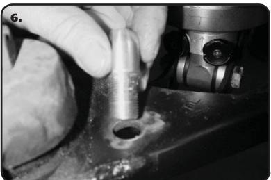
**6.** Insert the Aluminum Adapter into the sway bar hole in the control arm. Install a 5/8" Star Washer and 5/8"-18 Nylok on the Adapter. The Adapter needs to be aligned with the REAR control arm tube while tightening, refer to Diagram "7" for reference.
