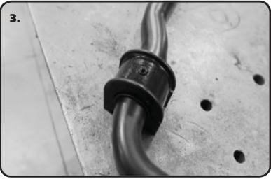
**3.** Open up the Poly SwayBar Bushings and install them over the Delrin Sleeves.
