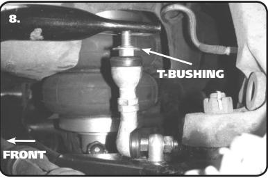
**8.** Insert the stud of the 90 degree end of the PosiLink into the Aluminum Adapter with the stud pointing to the rear of the car. Install a M10-1.5 Nylok Nut on the threads and tighten. Install a T-Bushing on the threads of the straight PosiLink with the LARGE diameter toward the PosiLink. Do this for both sides.
