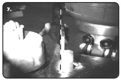
**7.** Align the FLAT of the Aluminum Adapter with the REAR tube of the control arm. Tighten the 5/8"-18 Nylok Nut.
