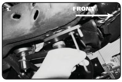
1. Attach the Adapter Plate to Frame positioned with the 3/8"-16 Stud to the Front of the Car and the Rear Hole aligned with the Rear OEM Hole. The Adapter Plate is attached to the Frame using a Flat Head Bolt and Red Loctite. The OEM Threaded holes can be either, 5/16"-18 or 3/8" -16, hardware is supplied for each. Apply Red Loctite to the proper Bolt and insert it through the Adapter. Thread the Bolt into the Front OEM Hole and tighten.
