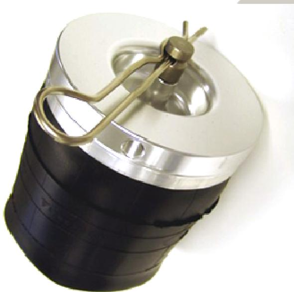
3. Apply thread sealant to a 90 degree air fitting and screw it into the top of the air spring.
