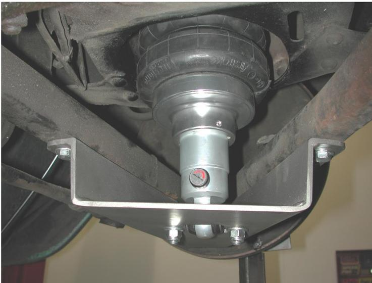
9. Swing the lower control arm up to the Shockwave. The T-bar will sit on top of the plate and is secured with two 5/16" x 1 1/4" bolts.
