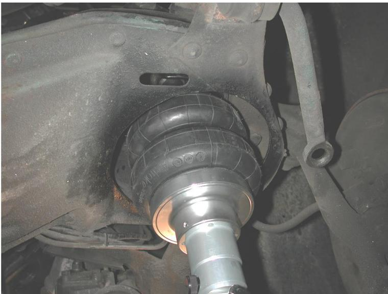
5. The bellow can be rotated separate of the shock to alter the air fitting location. It should point towards the inside of the car. The airline must also be routed at this time.
