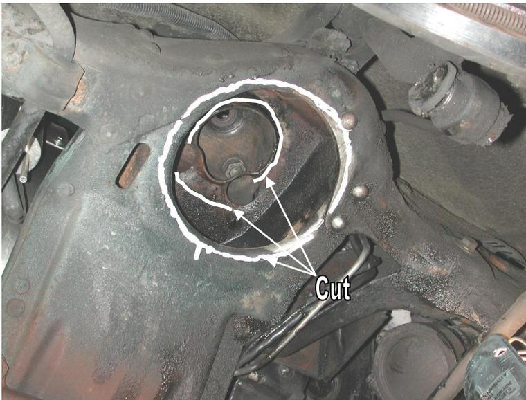
3. Due to the Shockwave bellow being larger than the coil spring you will have to open the coil spring pocket as shown by the white circle in the picture. You will also need to remove the lip of the coil spring retainer and cut between the large holes as shown in the picture. This is best done with a plasma cutter, cutoff wheel, or saw.
