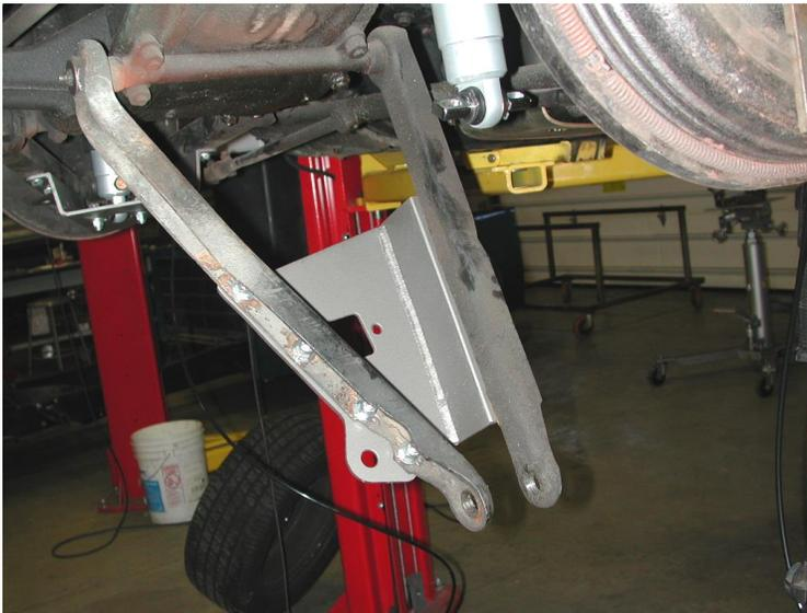
7. The coil spring plate on the lower control arm must be removed. It is attached by rivets, which must be ground off.
