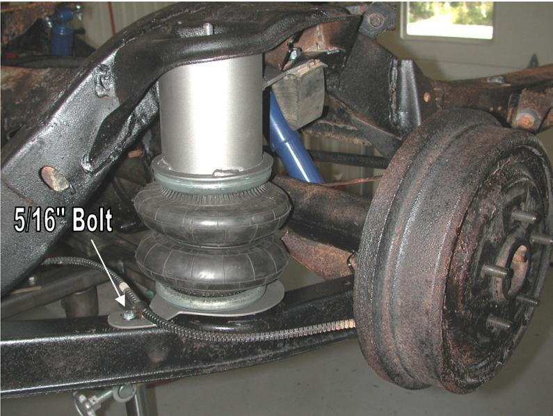
11. The hole in the tab on the lower mount will align with the parking brake cable clamp. It will be held tight with a 5/16" x 1" bolt, lock washer, and flat washer.
