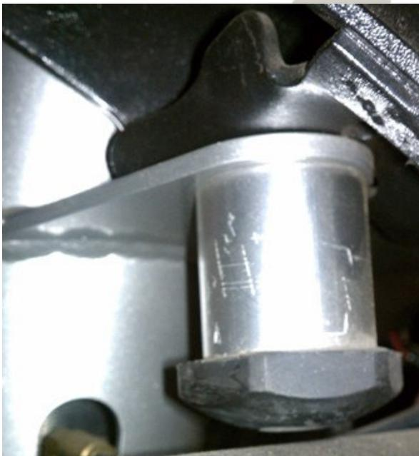
7. The stud should poke through the hole in the upper coil spring pocket. Some cars may not have this hole and it must be drilled. Fasten with a 7/16" Nylok nut and flat washer.
